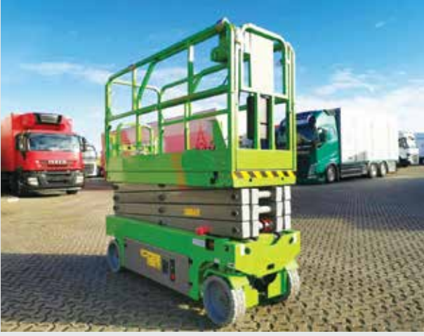
Tekerlekli makaslı personel platformu Wheel type scissor lift
