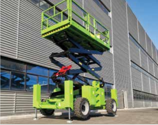
Arazi tipi makaslı personel platformu Rough terrain scissor lift specification
